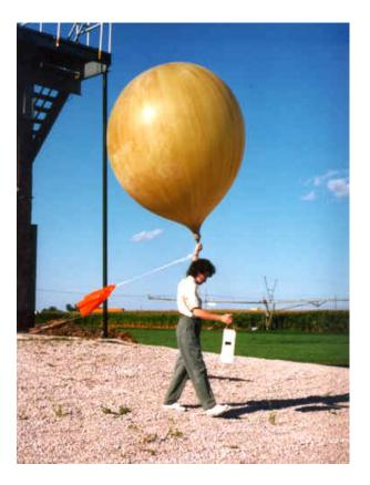
Figure 5. Radiosonde and Balloon Prior to Release (National Weather Service)
