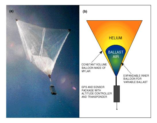
Figure 7. (Left) Ballasted Tetroon in Flight. (Right) Sketch of the "Smart" Tetroon Showing Primary Components. (Johnson, Carter, and Businger 1998, Businger et al. 1998)
