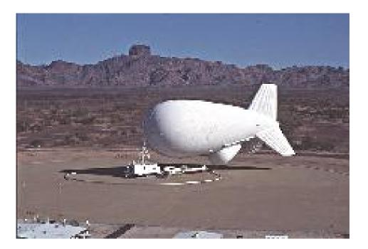
Figure 9. Tethered Aerostat Radar System Balloon-Borne Radar
