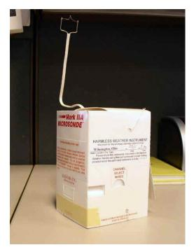
Figure 2. Radiosonde Instrument Package (National Weather Service)
