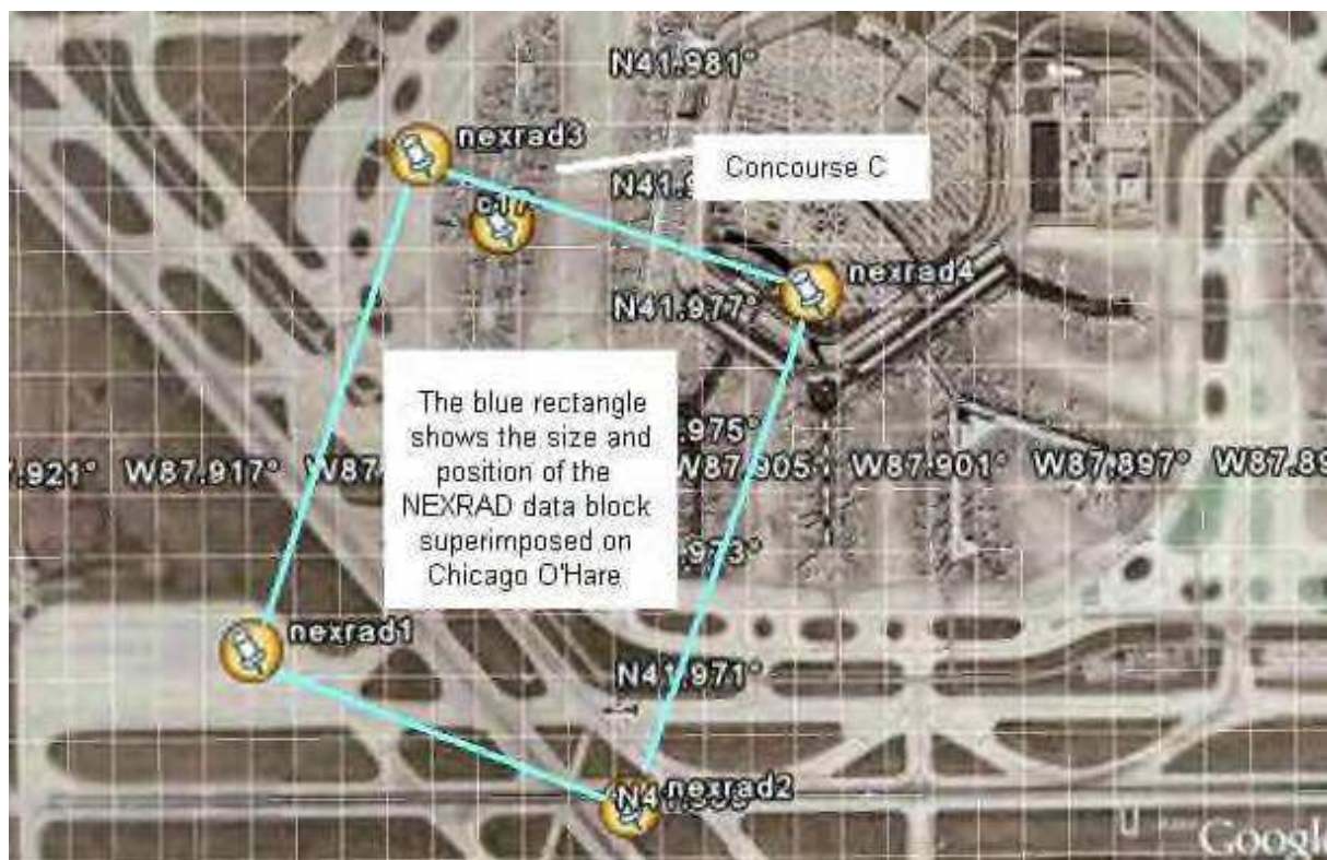
Figure 25. Footprint of the NEXRAD Radar Resolution Cell Superimposed on the Sighting Location (adapted from image supplied by James Smith)
