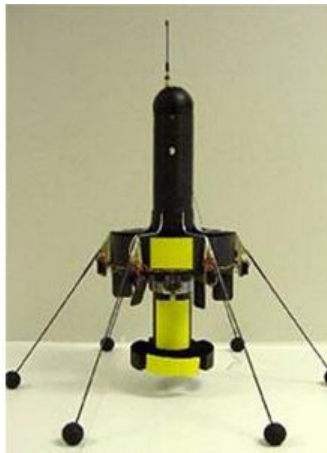
Figure 12. Micro Autonomous Systems, LLC, Heli Spy II (Diameter: 11"; Height: 27"; Velocity: 75 mph.; Endurance: 30 min.: Flies in vertical orientation but tilts 60 deg forward at top speed. )
