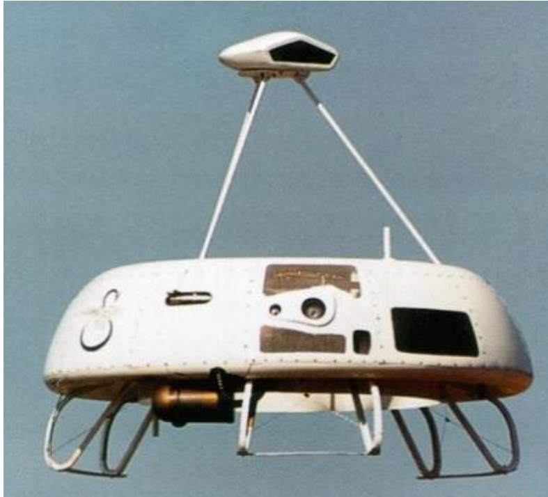
Figure 11. Sikorsky Aircraft Corp. Cypher II "Dragon" UAV (Diameter: 6' 2"; Height: 2'; Rotor Diameter: 4'; Max. speed: 145 mph. Range: 115 miles; Endurance: 2-3 hrs.)
