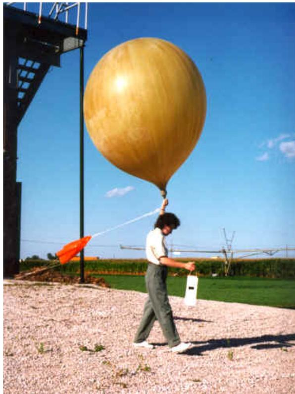
Figure 5. Radiosonde and Balloon Prior to Release
