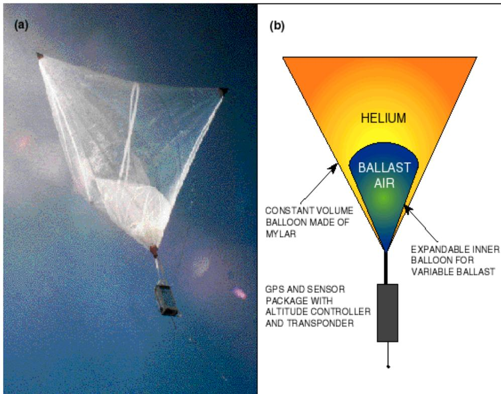
Figure 7. (Left) Ballasted Tetraon in Flight. (Right) Sketch of the “Smart” Tetraon Showing Primary Components. (Johnson, Carter, and Businger 1998, Businger et al. 1998)
