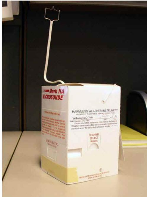
Figure 2. Radiosonde Instrument Package (National Weather Service)
